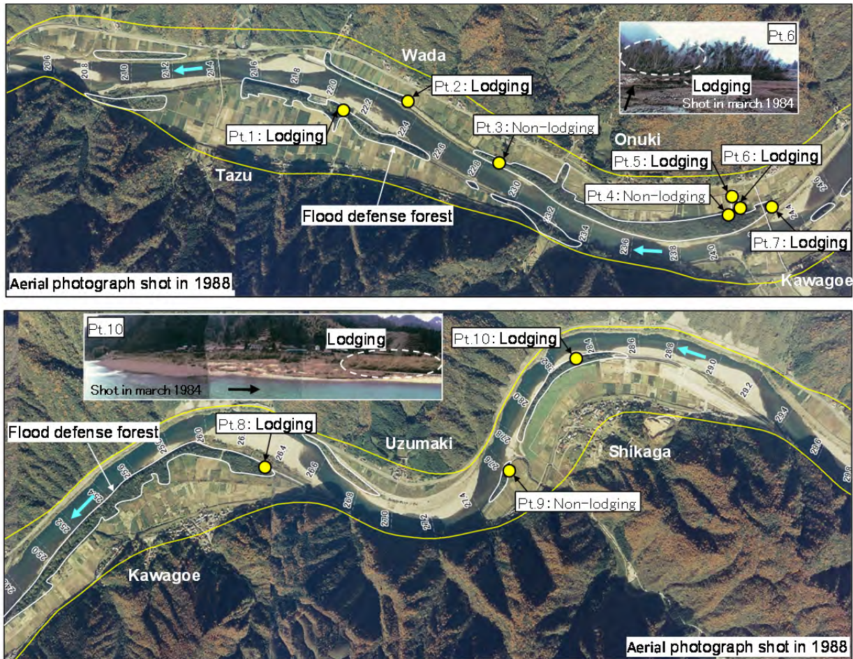
Figure 6. Aerial photograph after flood in July, 1988 and assessment of the flood defense forest after flood
