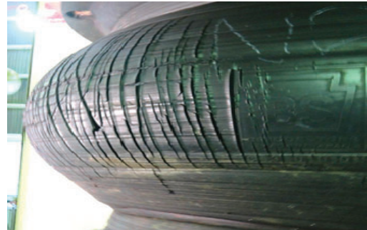
Fig. 4 Surface cracks under compression (3000H, 39 years)
