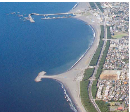
The Headland Plan in the Chigasaki area of Shonan beach (Kanagawa prefecture)
